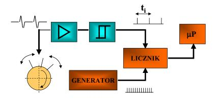
Fig.5. Structure of measurement tract used by diagnostic system SNDL-1b/SPL-2
