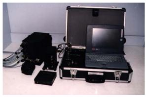
Fig. 3. S2-3a/P recording system for airborne tests
